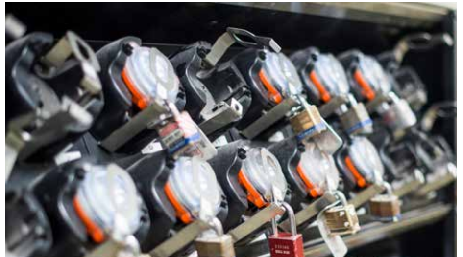
Recharging station for cap lamps
